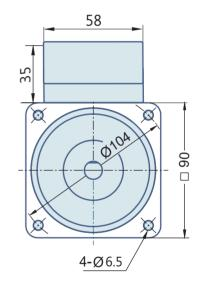
60 Watt: AC Geared Motor With Lead wires
