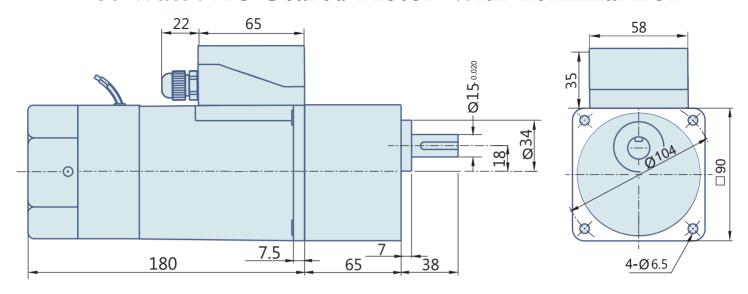
60 Watt: Round AC Induction Motor With Terminal Box
