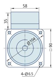
60 Watt: AC Geared Motor With Lead wires
