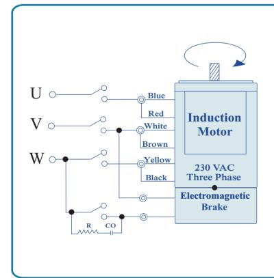
When Sw1 is switched ON, Electromagnetic Brake is released & motor starts rotating. When Sw1 is switched OFF then Electromagnetic Brake will be applied stopping the motor immediately & holding the load.
