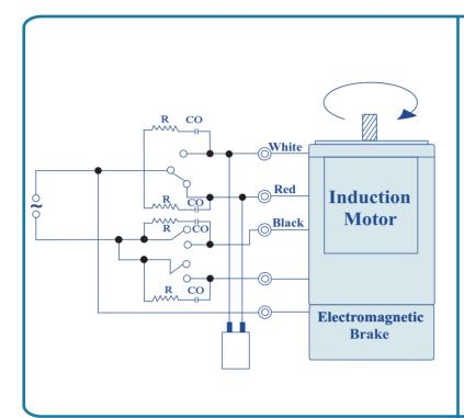
When Sw1 is switched ON, Electromagnetic Brake is released & motor starts rotating. When Sw1 is switched OFF then Electromagnetic Brake will be applied stopping the motor immediately & holding the load.
