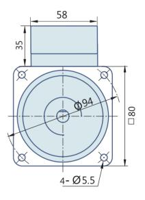
25 Watt: AC Geared Motor With Lead wires
