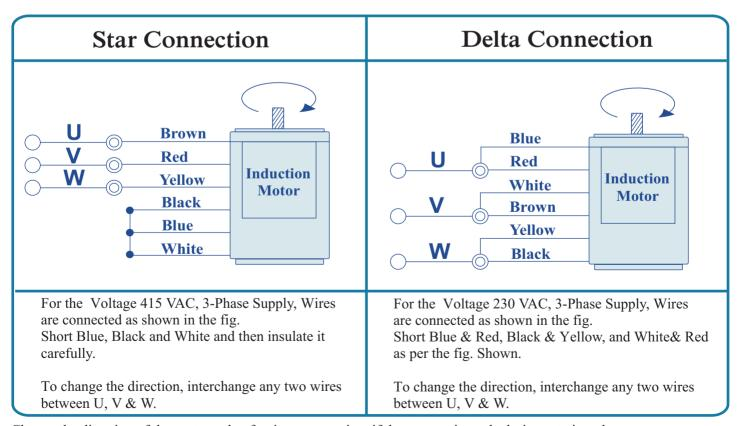
Change the direction of the motor only after it stops rotating, if the attempt is made during rotation, the motor may ignore the reversing command or change the direction after some time.
